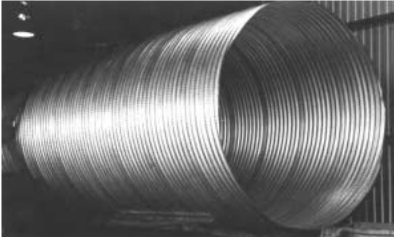
3000 mm (120 in.) diameter fully perforated pipe being fabricated on helical pipe mill.
